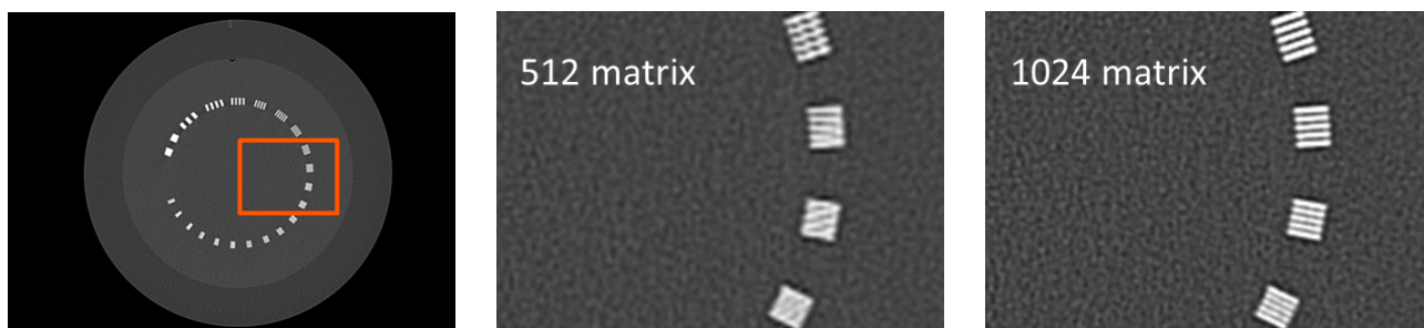
Fig. 1: Section from line pair high-contrast resolution phantom for kernel Br64 (50% MTF: 10.1 lp/cm), FoV of 300 mm, and different matrix sizes. Voxel size for 512 matrix is d = 300 \text{ mm} / 512 = 0.59 \text{ mm} and maximum spatial resolution that can be displayed is f_{\text{max}} = 10 \text{ mm/cm} / (2/lp * d) = 8.5 \text{ lp/cm} . For the 1024 matrix, f_{\text{max}} is 17 lp/cm.
